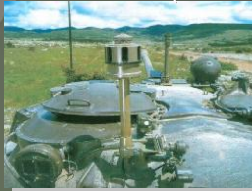
Laser irradiation warning system
